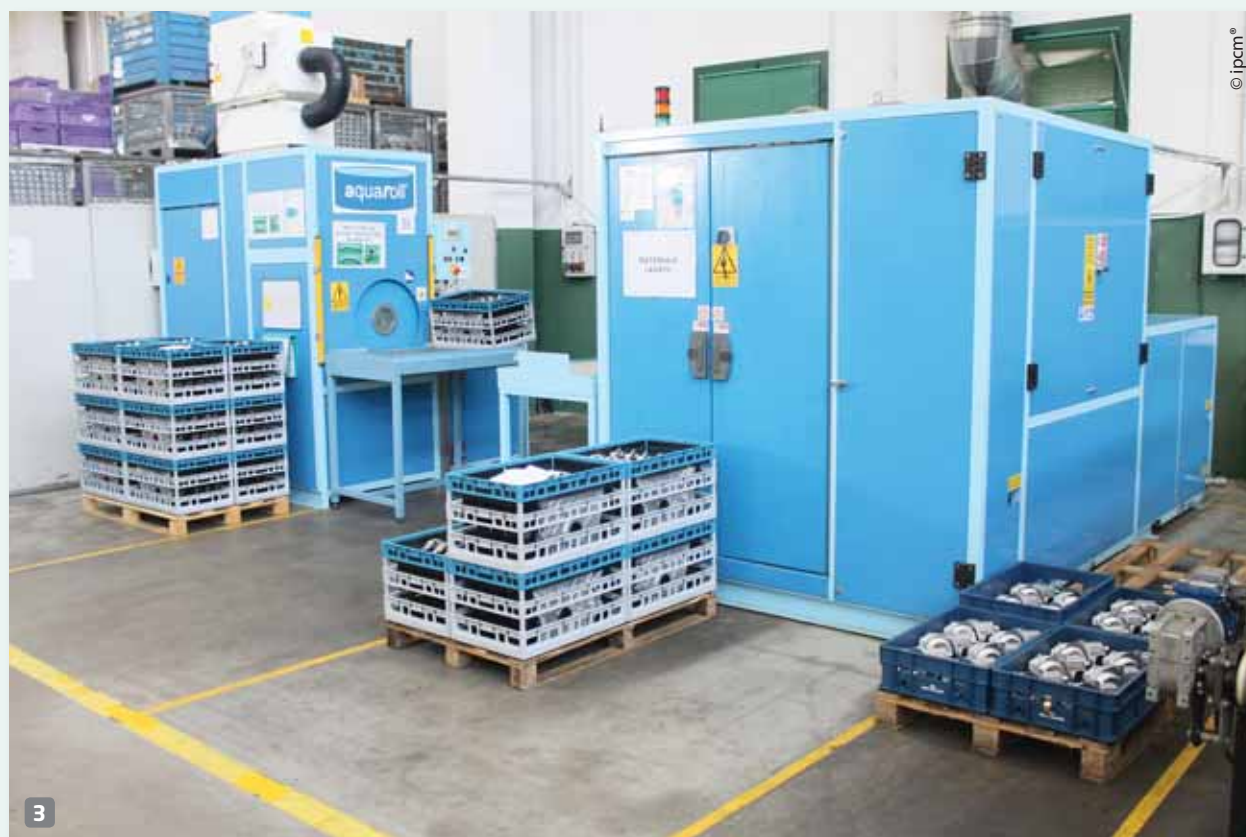
The two Aquaroll® systems installed at Sepam's premises by STS (Ravenna, Italy) for the bicarbonate-based deep cleaning of components.
